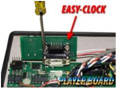
With the door hanging down locate and remove the green protective cover on the 9 pin connector Player board.
