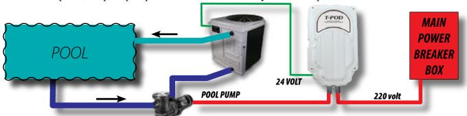
pool reaches temperature. Then both Heat Siphon and pump will shut off. To enable PumpJump™ just PRESS BOTH KEYS once and the blue LED will light indicating it is in PumpJump™. Repeat keypress to disable it.
