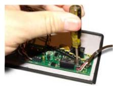
Loosen the set screw on the two POD terminals on the Player board. Insert the red and white wires into the POD terminals and screw down the set screws Pull on the wires to make sure they are securely fastened to the Player board.
